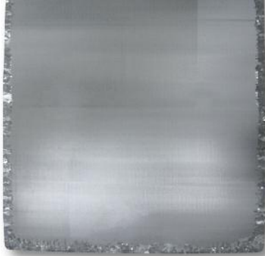
Typical Mono 2TM seed plate, which initiates uniform crystal growth of mono-crystalline ingots
