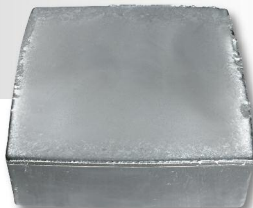
Mono 2 ™ ingot with monocrystalline brick structure
